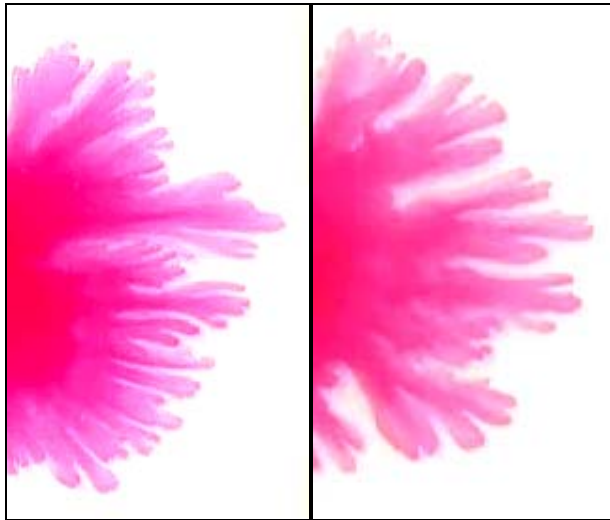
(a) Kerosene into light mineral oil – 1 cc/min
